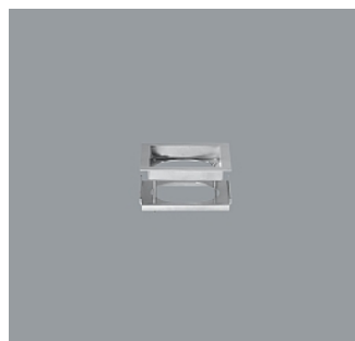
33786.000 Mounting frame To cover the floor aperture. Mounting in hollow floor. Stainless steel. Clamp extension 19-65mm. Weight 0.42kg
